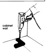
To mount anti-tip bracket to concrete or ceramic floor, use a masonry drill bit to drill 3/16" holes at each mounting screw location. Tap plastic anchors into mounting holes in floor with hammer.
